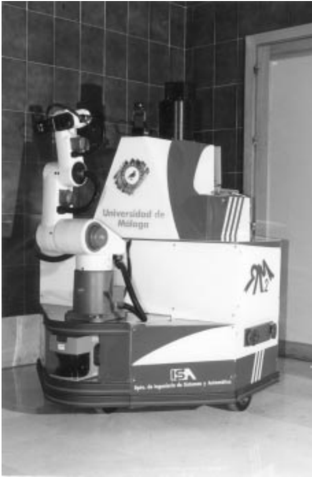
Fig. 2. The RAM-2 mobile robot. The METAL-A* algorithm has been implemented and tested in this platform for global path planning.
